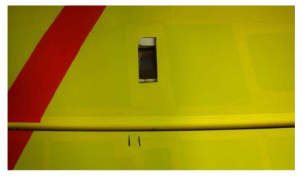
Cut servo hole and Use epoxy to install aileron horns as shown
