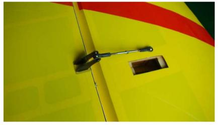
Attached servo extensions to aileron servos, Use the string install in the wing to pull the servo wire through the wing
