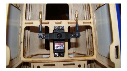
Crimp the servo end of the cables first, the cables cross once inside the fuselage to form an "X"  $\,$
