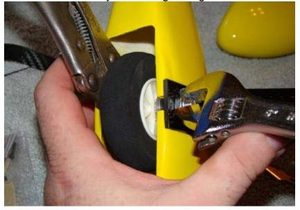
Repeat for other side, Install the wheel cover, and fix it up to landing gear with screw.
