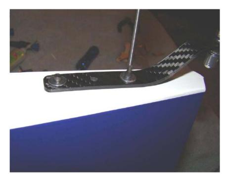
Apply epoxy into hinge hole of the rudder Use glue to fix up rudder horns.
