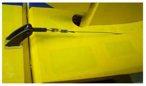
Install the rudder servo, servo, and hall links with locking nuts as shown
