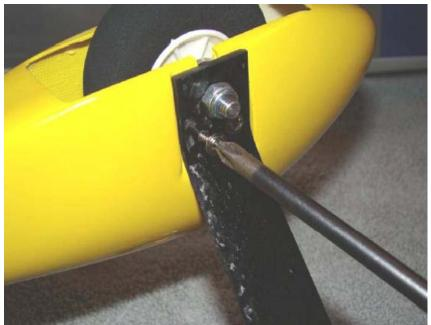
Fix up the landing gear on the fuselage bottom with 4 screws.
