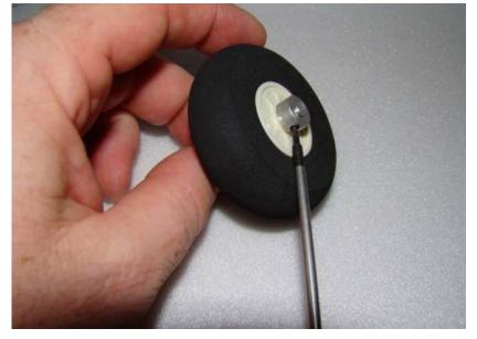
Slide on wheel/axle assembly into a wheel pant, and install the wheel assembly on the landing geat leg, Tighten the locknut as shown to secure the assembly onto the gear leg
