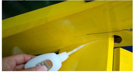
Hinge the elevators onto the horizontal stabilizer
