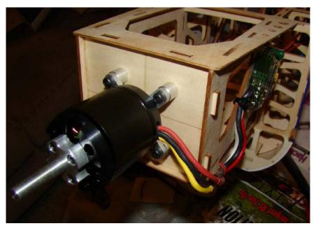
Drill a small hole, Fix the cowl with screw as the show.
