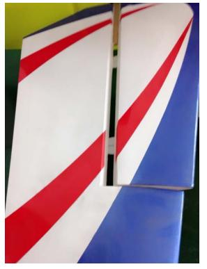
Install the elevator, Before installing the ekevator with the slot which accepts the joiner, practice fitting it once, the joiner is very tight in the slot
