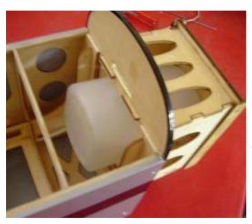
Install the fuel tank into the fuselage, and fixup it with belt.
