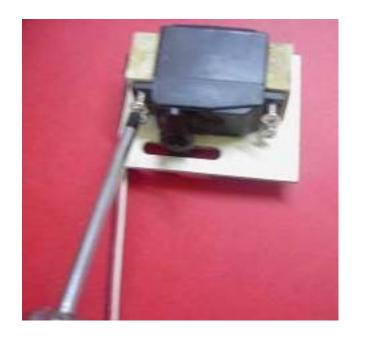
Insert the servo in the middle of two woods, then fix two TP screws on each side.
