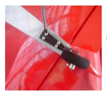
Fixup the tail wheel to the rudder with four TP screws.
