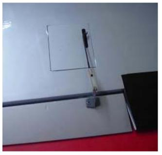
Insert the servo to the prepared servo hole then fix it with four screws . Connect tri-horn and servo with pushrod.
