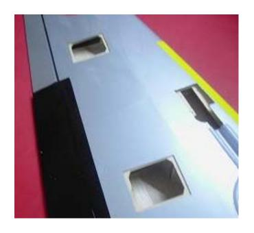
Cut the servo holes and retractable wheel hole under the main wing .
