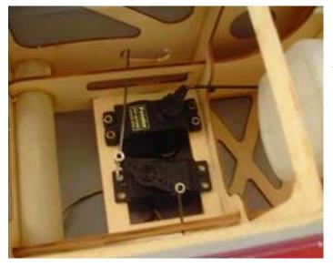
Assemble retractable wheel servo and throttle servo as shown.
