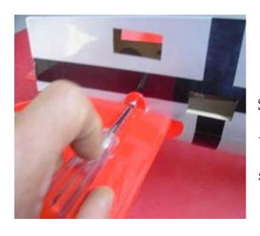
Screw the stabilizer to the tail fuselage with one 3\*12 screw on each sides.
