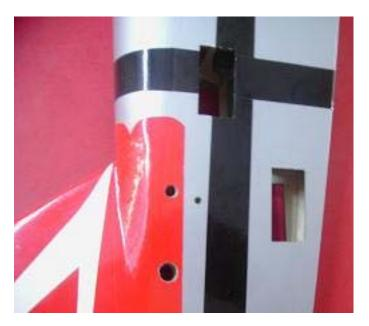
Find out the holes on the tail fuselage as shown.
