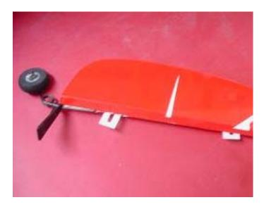
Insert the tail wheel landing gear into the rudder.
