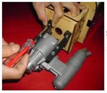
Screw the engine mount to the firework as shown.
