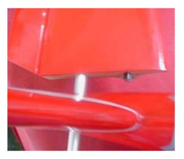
Insert the Aluminium bolt through the tail fuselage.
