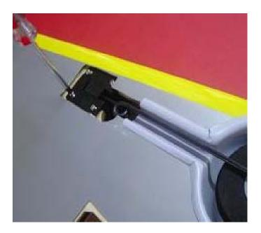
Fixup the retractable landing gear series with four TP screws.
