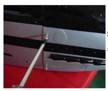
Screw the cowling with four TP screws as shown.
