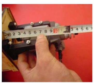
Measure the distance from firework to airscrew is 128MM.
