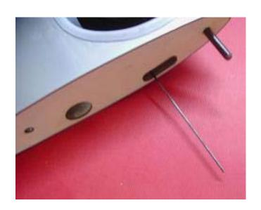
Assemble the retractable pushrod, then pull out it.
