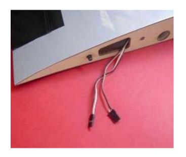
Put the servo into the hole and pull out the servo extension from main wing.
