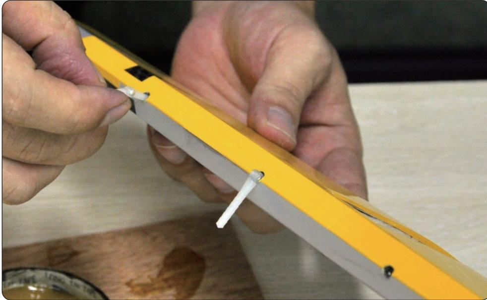
2. Cut out the holes on the fuselage of both sides.
