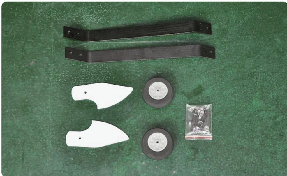
3. Use screw to connect the landing gear, wheel pant, nut and wheel in turn, and finally use a lock nut to lock them.
