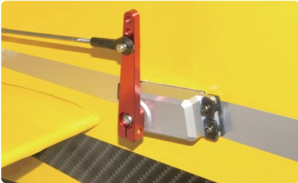
8. Install the ball links onto the servo arm and the control horn with stainless push rod supplied.
