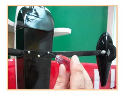
Install the main landing gear with the bolts provided and use blind nuts already installed and use blue Loctite on the mounting bolts
