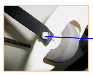
Install wheel pants with two mounting bolts.
