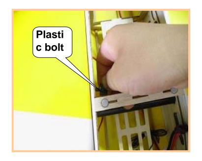
Mounting the wings with plastic bolts on both sides.
