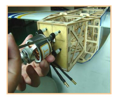
Install the motor to the four adapter and use screws to lock motor and adapter.
