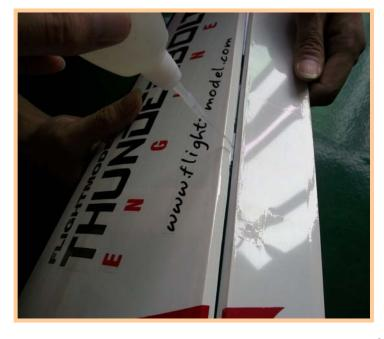
Connect the aileron and the main wing by hinges. Be sure to apply instant type glue to both sides of each hinges.
