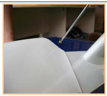
Use the TP screw and pads to lock the cowling.
