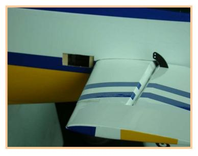
Find and cut the hole for stabilizer assembly and rudder servo .
