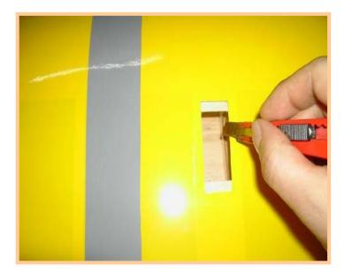
Cut the servo holes on the bottom of the main wings.
