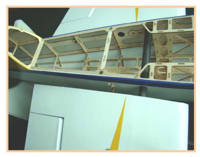
Find out the holes in each sides of fuselage, then remove the covering. Insert the carbon joiner in place, then put on wings.
