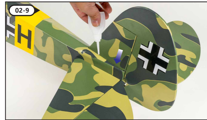
垂直尾翼插入机身尾部，调整使其与机身垂直后，连接处用CA胶水粘固。 Insert the vertical tail into the rear of the fuselage, adjust it so that it is perpendicular to the fuselage, and fix the joint with CA glue.
