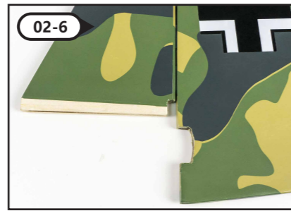
垂直尾翼安装完成后，用美工刀切除与机身结合面的蒙皮。 After the vertical tail is installed, use a utility knife to cut off the film of the joint surface with the fuselage.
