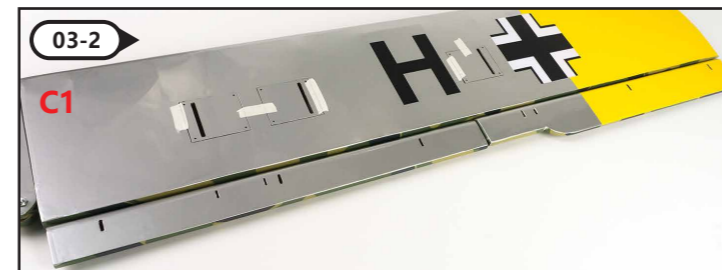
把襟翼，副翼如上插入机翼末端预留槽，通过纸合页连接，并在连接处用CA胶水粘固。粘完后确保襟翼和副翼可以自由摆动。 Insert the flaps and ailerons into the reserved slot at the end of the wing as shown above, connect them with paper hinges, and use CA glue at the connection. Make sure flaps and ailerons can swing freely after sticking
