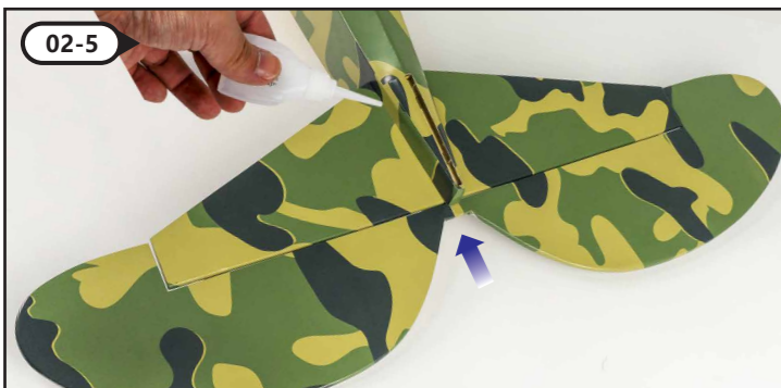
把尾翼安装到机身尾部，调整到平行于机身，连接处用CA胶水粘固。 After mounting the tail wing to the rear of the fuselage, adjust it to be parallel to the fuselage, and fix the joint with CA glue.
