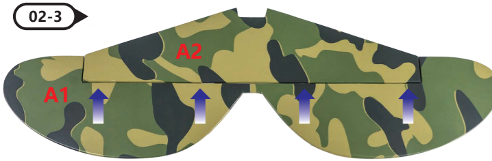
把升降舵、转向舵和尾翼通过纸合页连接，连接处点入CA粘固，并保持舵面可以自由摆动。 Connect the elevator, steering rudder and tail wing by paper hinges, put the CA glue at the joints, and keep the rudder surface free to swing.
