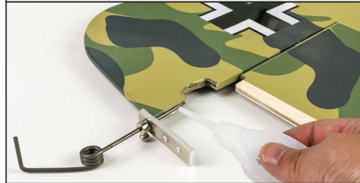
弯折好的尾轮组插入尾翼，用大量CA胶水粘固。 Insert the bent rear wheel set into the tail wing and fixed with a large amount of CA glue.
