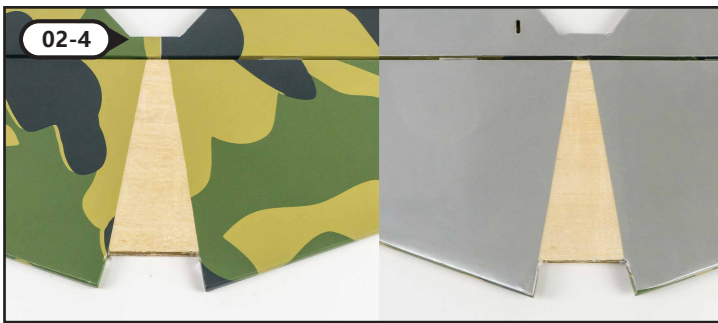
参考尾翼和机身尾部的结合面，用美工刀切除结合面的蒙皮。 With reference to the joint surface of the tail wing and the fuselage tail, use a utility knife to cut off the film of the joint surface.
