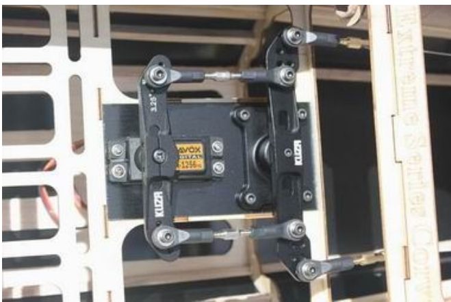
12. The EXTRA also provides pull-push style for rudder. Below is picture of pull-push style linkage set.
