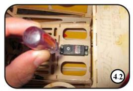
4.Drill 1mm holes. Install the servo with the M2\*12mm tapping screws.
