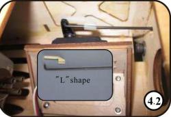
4. Remove pushrod from throttle arm on carburetor and cut throttle pushrod to length.. Use a L bend to connect the push rod to the servo arm.
