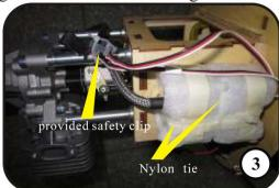
3. Thread nylon tie through mounting holes. Mount the engine ignition module using nylon tie as shown. Use the provided safety clips to secure the ignition and engine trigger line.
