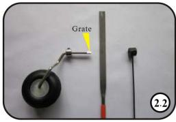
2. Install the wheel to the steel wire with wheel collars. All wheel collars should be secured with Blue Loctite. Grate the end of the steel wire with a
