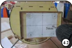
4. Drill four 5mm holes and a 5mm pushrod exit hole on the firewall.
