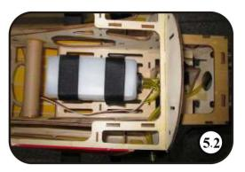
5. Drill a 6mm hole on the bottom of the fuselage. Let air line pass through the hole. Tighting the line with nylon tie will help to prevent lead from drawwing back inside of fuselage during flying. Retight the tank with the velcro tie after the fuel lines are all right.
