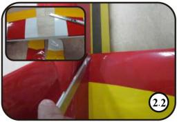
2. Mark the stab with a pen when the stab is symmetrical. Trace around the fuselage with a knife and remove the covering below to expose the board. Take care not to scratch the board.
