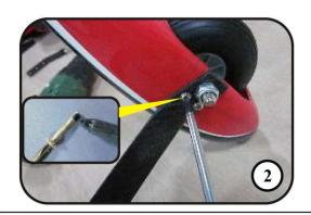
2. And then install the wheel pant with two M2. 5\*12mm screws.
