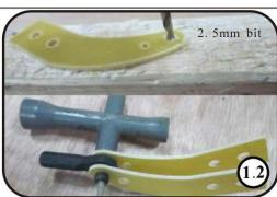
1. Scuff the horns with sand paper to ensure a good glue bond. Drill 2.5mm holes in the horns and install the M2.5mm ball link with the screw.
