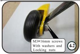
4.Install the inner wheel collar on the axle. Tighten the wheel collar in place. Adjust wheel collars in or out until wheel turns freely.
