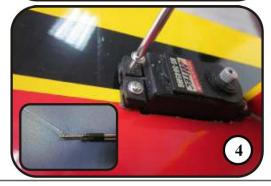
4.Install servo with M2\*12mm servo mounting screws. Use a drop of thick CA glue on each screw to prevent screws from loosening due to vibration.
