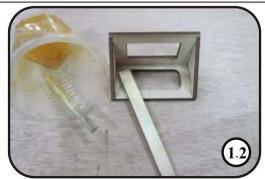
1. Drill 1mm holes in the throttle servo mounting and epoxy it.
