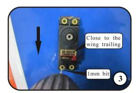
3.Drill 1mm holes for the servo mounting screws. Position the servo with the servo label closest to the wing trailing edge.
