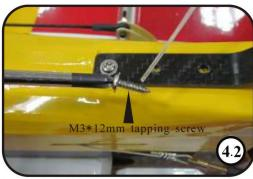
4. Use the tail wheel bracket as a template and drill 2mm holes. Install the tail wheel bracket with three M3\*12mm tapping screws.
