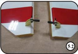
5. Install the two horns with M3\*16mm screw and locking nut. Apply 30 minute epoxy inside the pre-cut slots and coat the horns with epoxy, Insert them into the pre-cut slots.
