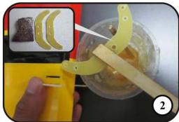
2. Scuff the middle of horns with sand paper to ensure a good glue bond. Apply 30 minute epoxy inside the precut slots. Coat the horns with epoxy. Insert them into the pre-cut slots.
