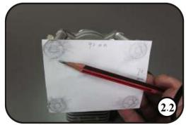
2. Tape a piece of 90\*70mm paper to the side of the engine mounting with the double-sides tape. And stamp for the engine mounting on the paper with a pencil. Position the pushrod exit hole also.
