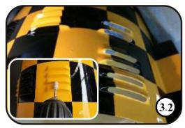
3. Use a rotary cutting tool and sanding drum to cut out the openings in the cowl. The shape and size of open pore depends on the type of the engine.
