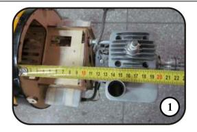
1. Measure the distance between the fuselage and the ignition plug (and exhaust).
