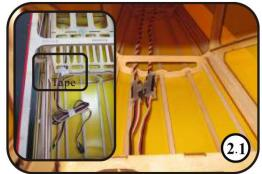
2. Run the extension lead through the fuselage to the receiver. Taping servo lead to the fuselage will help to prevent lead from dropping back inside of wing panel during flying.
