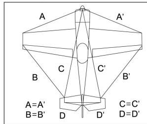
Adjust the aircraft and make sure both sides are symmetrical. Like the diagram shown. So that the plane is ready for flight.
