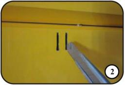
2.Pre-hinged control surface is ready to fly. Remove the covering below to expose the pre-cut slots with a knife...
