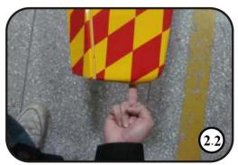
2. For CG proper position should be at 27%MAC. This recommendation balance point is for your first flights.
