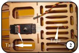
2. Position the servo with the servo label toward the fuselage tail. Fasten the servo wire with the tape.
