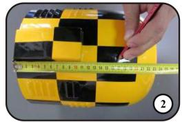
2. Measure the same distance on the cowling and mark it.
