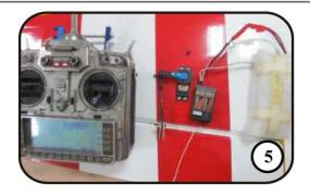
5. Mount the servo arm and the extension arm with M2\*8mm screws and locking nuts as shown. Then turn on the transmitter and plug the servo into receiver. Ensure the channel is neutral. Install the servo arm facing toward the wing tip. Position the servo arm 90 degrees to the servo.
