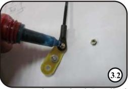
3 Thread the 2mm ball link half way onto the pushrod. Install the pushrod to the throttle arm with M2\*8mm screws.
