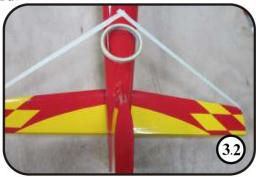
3. Coat the horns with epoxy. Insert them into the fuselage again. Make sure the stab is symmetrical and fasten it with the tape.
