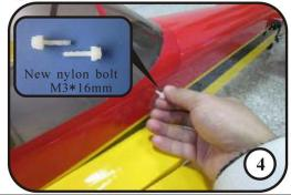
4.Install the canopy to the front of fuselage. Tighten the canopy with the M3\*16mm nylon bolts.
