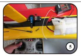
5. Turn on the transmitter. Make sure the servo is in the neutral position. Install the servo arm. Position the servo arm 90 degrees to the servo, and tighten the arm screw.
