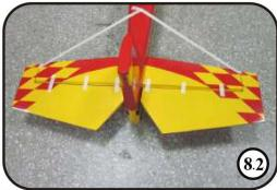
8. Coat other sides of the hinges with the epoxy and insert them into the stab hinge-holes. Check you have full elevator deflection before fasten with tape.
