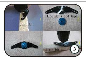
3.Drill 2.5mm holes in the AL long arm for installing 2.5mm ball links and screws.Drill 2mm holes in the servo arm and mount it with M2\*8mm screws and nuts.
