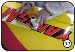
3. Using a piece of cloth. Spread decal smooth and remove all excess application fluid. Stick the decal to the wing cover while tearing out the decal as shown. Stick other decal to the fuselage or the part you want to decorate.
