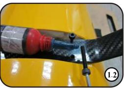
1.NOTE: the correct edge in mounting. Install the landing gear in the pre drilled holes with the supplied M4\*25mm hex socket screws. All screws should be secured with Blue Loctite.Don't over tighten and crack the carbon fiber.
