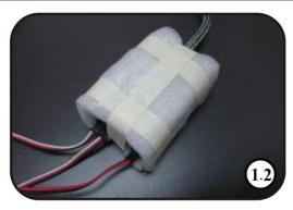
1. Trim a piece of foam rubber to the ignition module. Make the pad slightly larger than the ignition module. Bundle the ignition with tape as shown.
