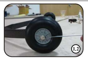
1.Install the inner wheel collar on the axle. screw and tighten the wheel collar in place. Adjust wheel collars in or out until wheel turns freely.
