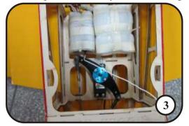
3. Adjust the battery back location. The CG can be moved around later to fit your personal taste.
