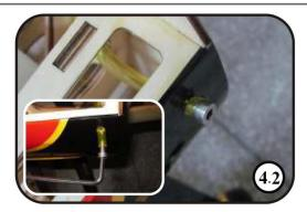
4. Drill a 6mm hole on the side of the fuselage. And then let 6mm pumping fuel line pass through the hole. Install the M5mm screw to seal the fuel line.
