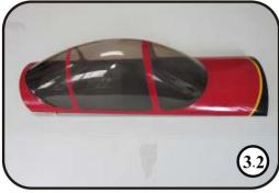
3. Us thin CA to secure front hatch hold down dowels. It is highly recommended you apply thin CA glue to the front hold down dowels. This is a High vibration area and can loosen the front dowels.
