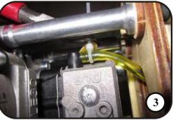
3. Install the engine fuel line to the carburetor tube. Tight the fuel line with nylon tie.
