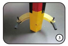
3. Install the ball link with M2. 5\*16mm screws and locking nuts. Tightening the nuts recommended. Wipe away glue with rubbing alcohol. Make sure the horns are correctly aligned and symmetry before the apoxy has cured.
