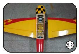
5. Slide the wing tube in the fuse wing tube sleeve.
