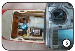
5. Turn on the transmitter. And then install AL long arm on the servo. position the servo arm 90 degrees to the servo.
