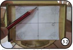
3. Draw the center-lines with a pencil as shown. Stick the tamplate paper onto the firewall with the center-lines coincident.
