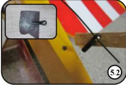
5. Drill 4mm holes in the bottom of the rudder. Scuffing the ball link with sand paper to ensure a good glue bond is suggested before gluing. Make sure the ball link hole is parallel to the rudder. Apply 30 minute epoxy inside the 6mm hole and coat the hinges with epoxy, Insert the ball link into the hole.
