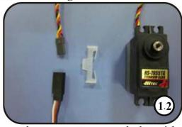
1. Remove the covering below to expose the pre-cut sevro hole with a knife. Use the provided safety clips to secure the servo and servo extension leads.
