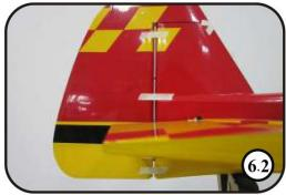
6. Insert them into the stabilizer hinge-holes. Check you have full rudder deflection before fasten with tape.
