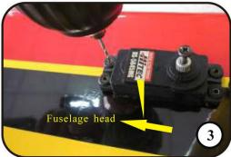
3. Position the servo with the servo label toward the fuselage head. Drill 1mm holes for the servo mounting screws using the long aiguille.
