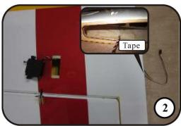
2. The covering of the servo location had been remove as shown. Put the end of the servo extension in the servo location. And then pull the extension lead through to the root of the wing. Taping servo lead to the inside of the wing panel will help to prevent lead from dropping back inside of wing panel during transportation.
