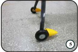
5. Repeat above steps for other wheel and wheel pant. Final landing gear installation shown below.
