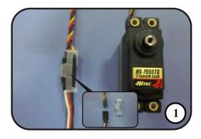
1.Use the provided safety clips to secure the servo and servo extension leads.
