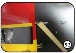
5. Insert the them into the rudder hinge-holes. Watch the hinges direction. Coat other sides of the hinges with the epoxy.
