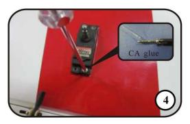
4. Use a drop of thick CA glue on each screws to prevent tapping screws from loosening due to vibration. Install servo with M2\*12mm tapping screws.
