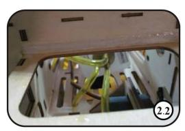
2. The tank bottom and cabin connect to the tank places had originally sticky connected to the VELCRO tie. Untie the velcro and install the fuel line on the copper pipe.
