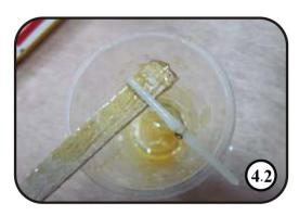
4. Scuff the hinges with sand paper to ensure a good glue bond. Apply 30 minute epoxy inside the hinge-holes and coat the horns with epoxy.
