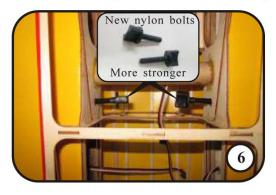
6.Install the nylon bolts to the wing blind nuts. Tighten snugly but do not over tighten. Slide the wings on the wing tube and plug in the aileron servo connectors.
