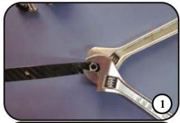
1. Install the carbon fiber tail wheel bracket with M5mm locking nut and M5 permanent seat AL screw.
