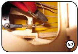
6. Mount the pre-installed ball link to the servo arm with the M2. 5\*16mm screws and the locking nuts. Remove any slack in the cables and crimp to secure. Crimp the brass swage tube with a crimping tool or pliers. Finally you can adjust the cable by loosening or tightening the cable connectors.
