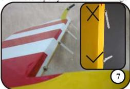
7. Insert the them into the elevator hinge-holes. Watch the hinges direction.
