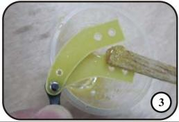
3.Apply 30 minute epoxy inside the pre-cut slots and coat the horns with epoxy, Insert them into the pre-cut slots. Wipe away excess glue with rubbing alcohol.
