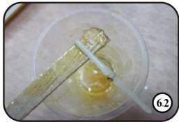
6. Scuff the hinges with sand paper to ensure a good glue bond. Apply 30 minute epoxy inside the hinge-holes and coat the horns with epoxy.
