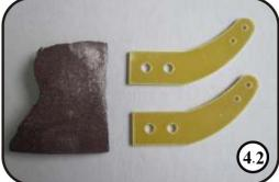
4.Remove the covering below to expose the pre-cut slots with a knife. Scuff the horns with sand paper to ensure a good glue bond.
