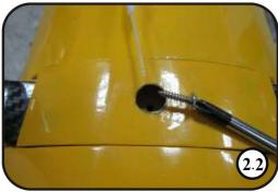
2. Remove the covering below to expose the holes with a knife and reinstall the landing gear hatch cover. Secure the M3\*12mm tapping screw with a drop of CA. The hatch cover maybe not included in some planes.
