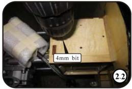
2. Position the ignition module on the side of the engine mounting box and mark the location of the nylon tie holes as shown. Use a 4mm bit to drill the ignition module mounting holes.
