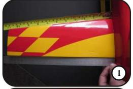
1. Insert the stab into the fuselage tail. Measure the stab to find the middle.
