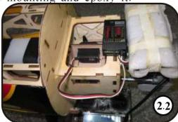
2.Mount the servo mounting with M2\*12mm tapping screws or epoxy. Turn on the transmitter. And then install the arm on the
