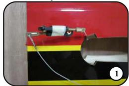
1. The rudder cables and couplers have been pre-installed.
