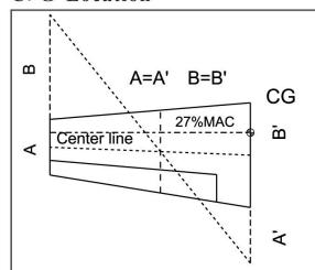
1. Measure the CG from the leading edge of wing against the fuselage.
