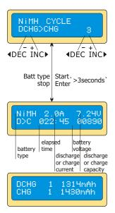
Set the sequence on the left and the number of cycle on the right. You can use this function for balancing, refreshing and break-in the battery. To avoid rising temperature of the battery, there will be a brief cool-offperiod that already fixed at 'User setting' after each charge and discharge process. The cycling number ranges from 1 to 5.
