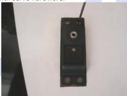
c. Next remove the servo and use thin C.A. glue to reinforce the threads. After the glue is dry reinsert the servo.
