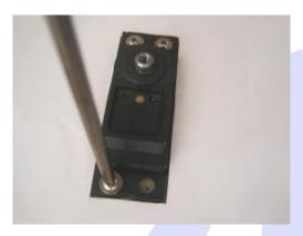
f. Using the supplied pushrod screw a ball-link onto each end.
