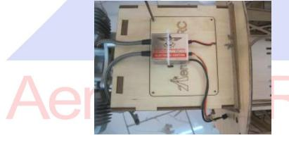
8. Mount the engines ignition to the motor box on radio foam to reduce vibrations.
