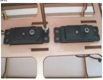
c. Using servo screws fix the servo in place, note the spline is towards the front of the plane.
