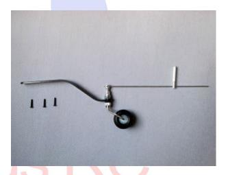
3. Before glueing in till mount be sure to slip tiller mount over tiller rod.
