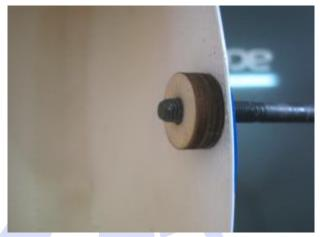
Next, insert the bolt from what will be the outside of the wheel pant; put one thicker wood spacer on to the axle bolt, followed by the wheel and one more wood spacer.
