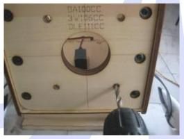
2. mount the engine with the stand offs to the bulkhead. Remember to use large washers on the inside to spread the load and use plenty of thread-lock.
