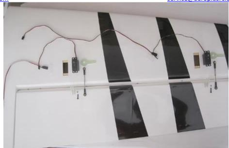
b. Now pre drill the servo mounts with a 1/16 drill bit, then secure the servo into the servo mount with servo hardware.
