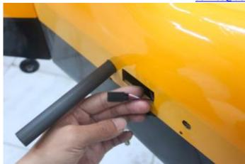
b. Connect the servo to the extension but be sure to use a servo clip or a piece of heat shrink to ensure it does not become disconnected during flight.
