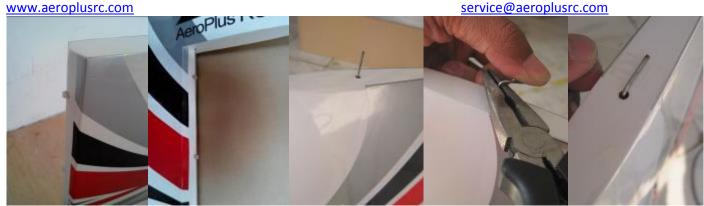
5. Glue the rudder horns in the rudder with epoxy; wipe off excess glue while it is wet.
