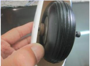
Install a lock nut onto the axle-bolt, followed by a washer.
