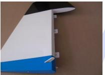
Sand the area on the horn that fits inside the rudders o the glue bonds better
