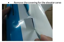
• Remove the covering where the elevator homs fit, use either a soldering iron or a sharp knife.
