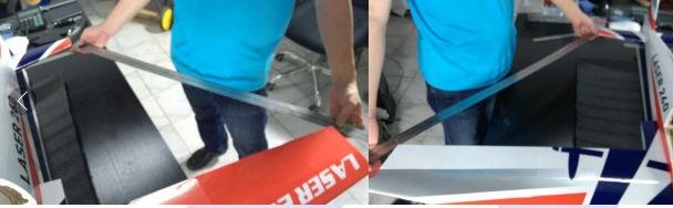
• Glueing – Once you think you are ready to glue, measure again. We recommend 2 methods for gluing. Either remove the covering on the area that is covered by the fuselage and glue with CA or epoxy, or leave the covering on and glue with thin cyno. Wicking in thin first, if a large gap is visible then use medium or thick. Remember to wick in small a mounts at a time keeping the plane level, this will ensure the glue stays where it needs to be.
