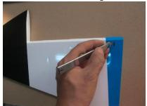
Test fit the rudder horns
