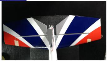
Remove the covering where the aileron horns are glued in place. Use either a soldering iron or a sharp knife
