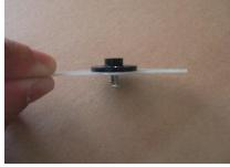
• Fit the rudder servo and drill holes using a fine drill for the servo screws, drop thin cyno into the holes to strengthen the wood.
