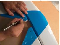
• The area on the horns that goes inside the elevator needs to be roughed up with sandpaper. This allows a better glue joint.
