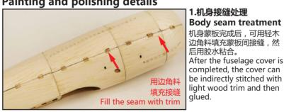
后用胶水粘合。 After the fuselage cover is
