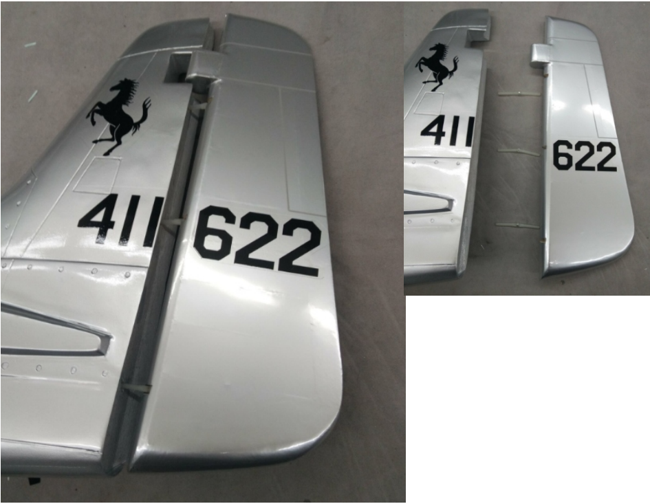
Connected fuselage and rudder by hinge, and use some AB glue or Epoxy glue to fixed it.
