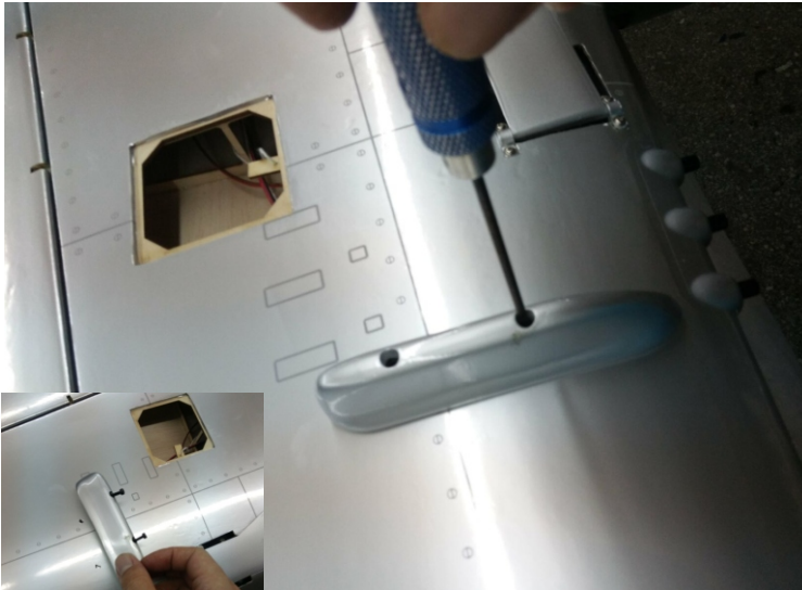
Fixed drop tank parts by screws.
