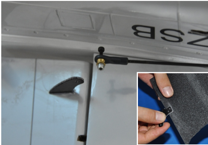
Put some AB glue or Epoxy glue to install elevator servo arm.
