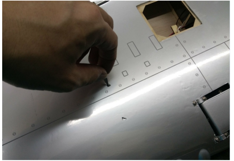
Open a hole for drop tank parts.
